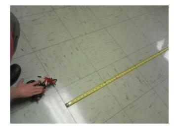
**Assessment:** Since the target distance is 10 ft, 11 ft would be recorded as a 1 ft amount of error. 9 ft would also be recorded as a 1 ft amount of error. A car that travels 10ft, but veers to the side 2 ft would be recorded as a 2 ft amount of error. Calculate the accuracy for each team and determine the order. Award points for  $1_{st}$  place through last place.
